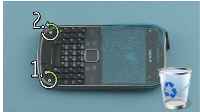
14) Unscrew the two Torx+ size 4 screws of the E-COVER. Do not use them again. Discard them.
