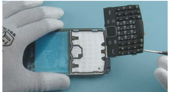
22) Remove the KEYMAT with tweezers.
