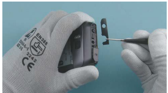
10) Remove the END CAP with tweezers.
