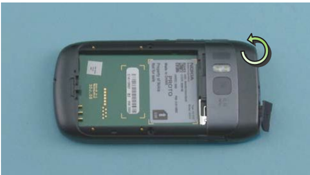
11) Unscrew the other top Torx+ size 4 screw and remove it with tweezers.
