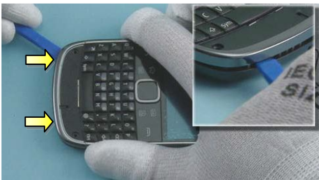
15) Use the SS-93 to release the shown clips of the E-COVER.
