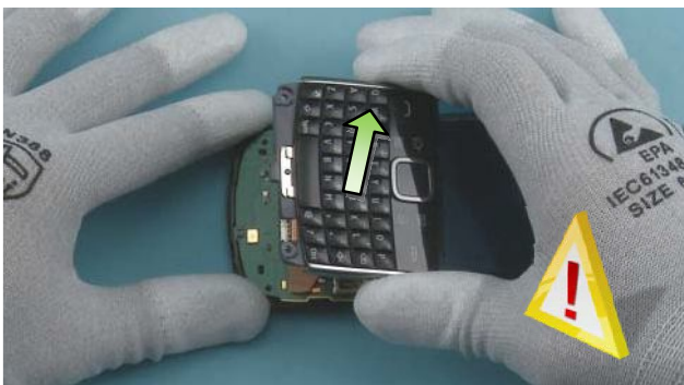
17) Lift up the WINDOW / TOUCH ASSEMBLY on the bottom side. Be careful not to damage the connector or components nearby!
