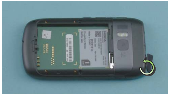
8) Unscrew the first top Torx+ size 4 screw and remove it with tweezers.
