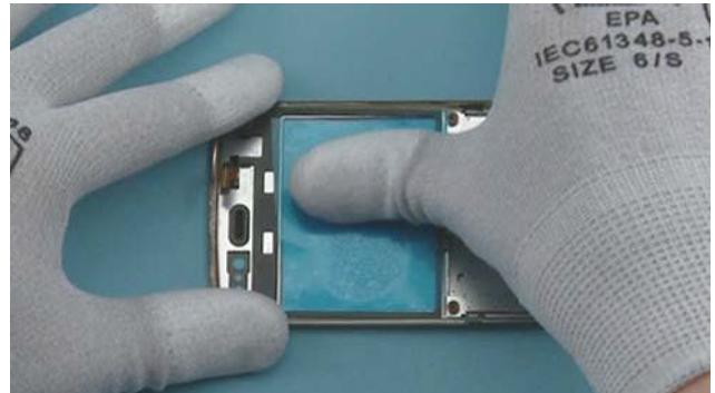
20) Protect the other side of the WINDOW / TOUCH ASSEMBLY with protective film.
