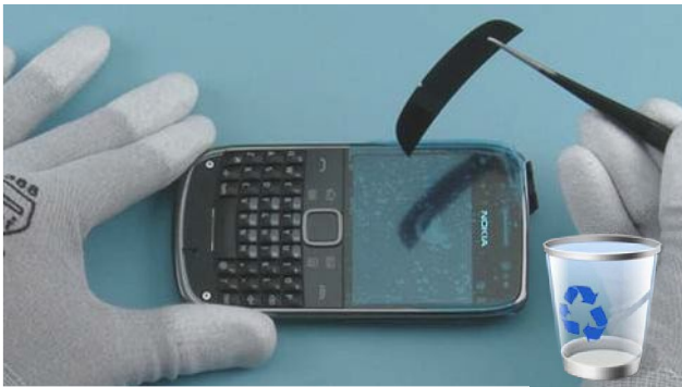
13) Remove the DECO PLATE with tweezers. Do not use it again. Discard it.
