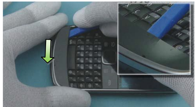
12) Use the SS-93 to lift up the DECO PLATE.
