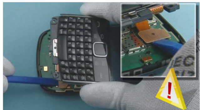
18) Open the WINDOW/ TOUCH ASSEMBLY connector. Be careful not to damage the connector or components nearby!
