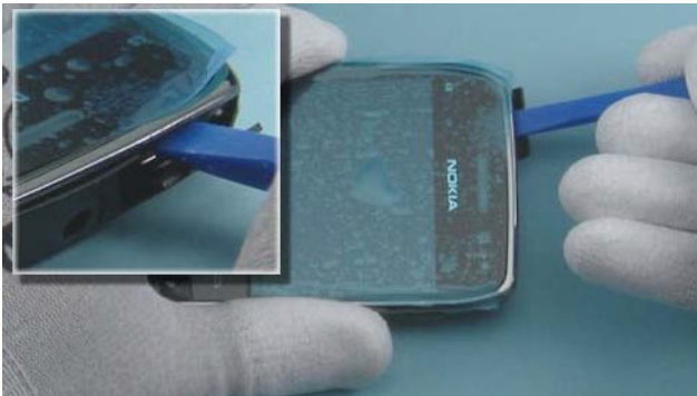
7) Use the SS-93 to open the SD door.
