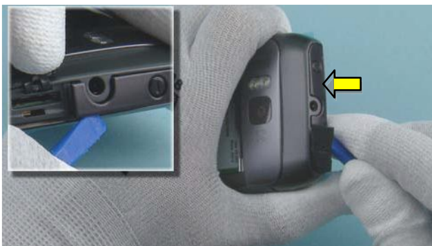
9) Open the clips of END CAP with the SS-93.
