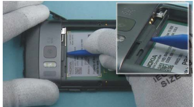
26) Push the SS-93 into the hole of the B-cover to release the ENGINE BOARD.
