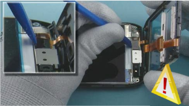
19) Open the touch panel connector and remove the WINDOW / TOUCH ASSEMBLY. Be careful not to damage the connector or components nearby!
