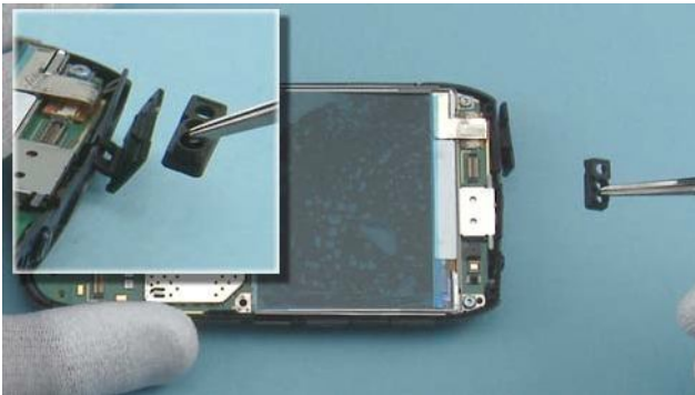
25) Remove the CAMERA BOOT with tweezers.
